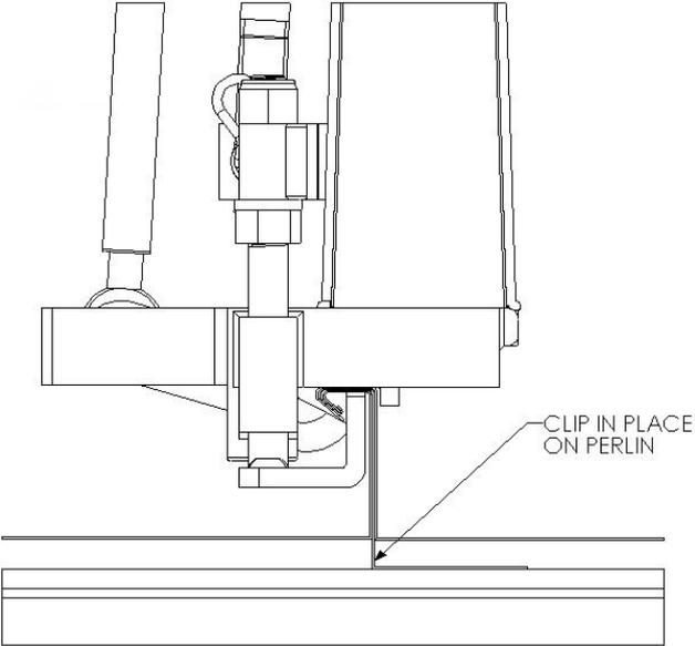
SEALOX 3 CRIMP HANDLE ACTUATION CRIMPS PANEL RIBS
